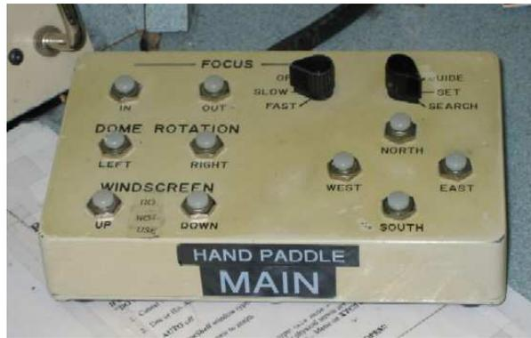
Figure 10—Main Hand Paddle Controls for Dome Orientation for Spectroscopic Flats
