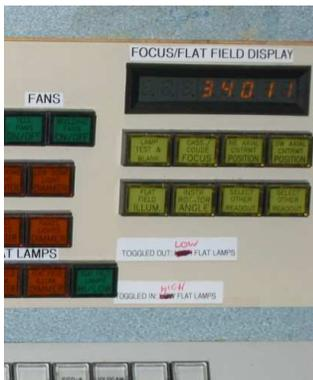
Figure 12—Close-up Photograph of FOCUS/FLAT FIELD DISPLAY CONTROLS.
